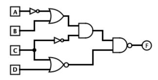
(B) Find a minimal implementation of the function below using only **2-input NAND gates**. *We will only accept circuit diagrams.* [6 pts]
