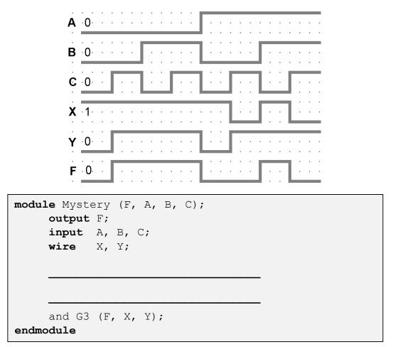
(B) Given the Verilog module Circuit below, assume that all gates (only 1- and 2-input) have a delay of 30 ns. If the values of inputs A and B first become known at t = 0 and output F is unknown at t = 0, at what time does F first become known? [3 pts]
