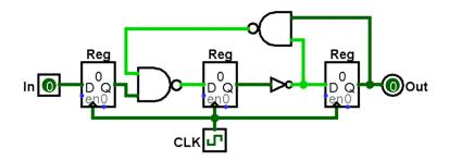
(A) Calculate the **minimum clock period** that will allow the circuit to function correctly. Make sure to *include units*. [3 pts]
