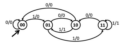
(A) What two 3-input sequences does this FSM "recognize" (*i.e.* when it outputs a 1)? [2 pts]
