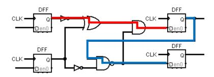
(A) Calculate the **minimum clock period** that will allow the circuit to function correctly. Make sure to *include appropriate units in your answer*. [3 pts]
