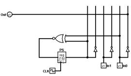
For both NS and Out: [1 pts] Truth table transcribed to K-Map correctly [2 pts] Correct simplification [1 pts] Correct circuit diagram  $Out = \overline{In_0}$  $NS = \overline{PS} \cdot \overline{In_0} + PS \cdot In_0$
