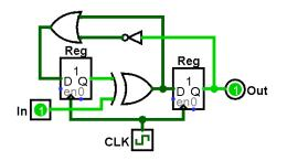
(A) Calculate the **minimum clock period** that will allow the circuit to function correctly. [3 pts]
