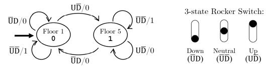
(A) How many total rows are in the truth table for the 3-way switch FSM? How many of the rows are filled with Don't Cares? [2 pt]
