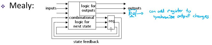
Input changes can cause immediate output changes
