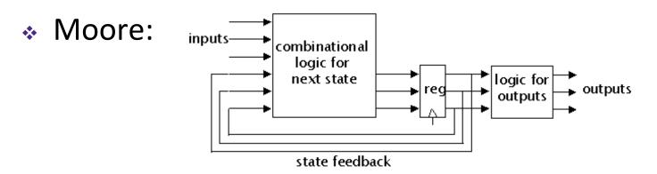
Outputs change synchronously with state changes
