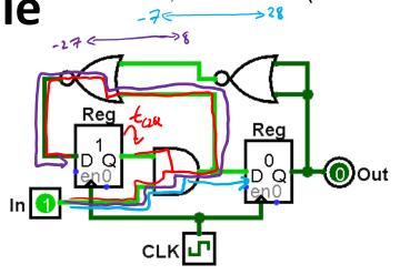
If In changes  $t_{CO}$  after each clock trigger, what is the minimum clock period we can use? crafical path(s) shown in red.
