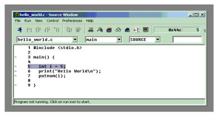
From the **Run** pull-down menu, select **Connect to target** in the mb-gdb window. In the Target Selection dialog, you can choose between the **Simulator** (built-in) and **Remote/TCP** (for XMD) targets.
