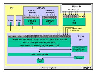
Figure 4-12: The Interrupt Service in the IPIF
