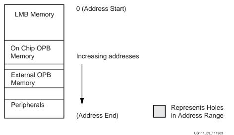
Figure 22-1: A Sample Address Map for a MicroBlaze System
