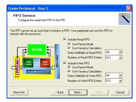
Figure 4-10: Configure Read/Write FIFOs
