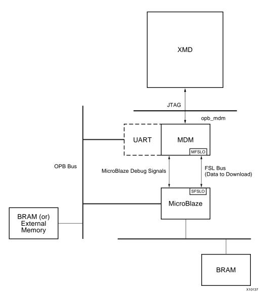
*Figure 13-5:* **MicroBlaze-MDM connection for Fast Download**
