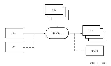
*Figure 6-3:* **Structural simulation model generation**
