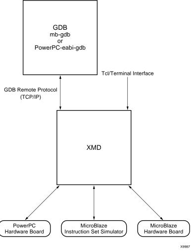
Figure 12-1: GDB Debugging Using XMD
