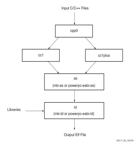
Figure 11-1: GNU Tool Flow
