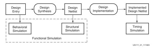
Figure 6-1: FPGA design simulation stages
