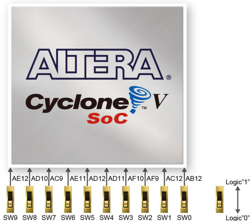
Figure 3-15 Connections between the slide switches and the Cyclone V SoC FPGA
