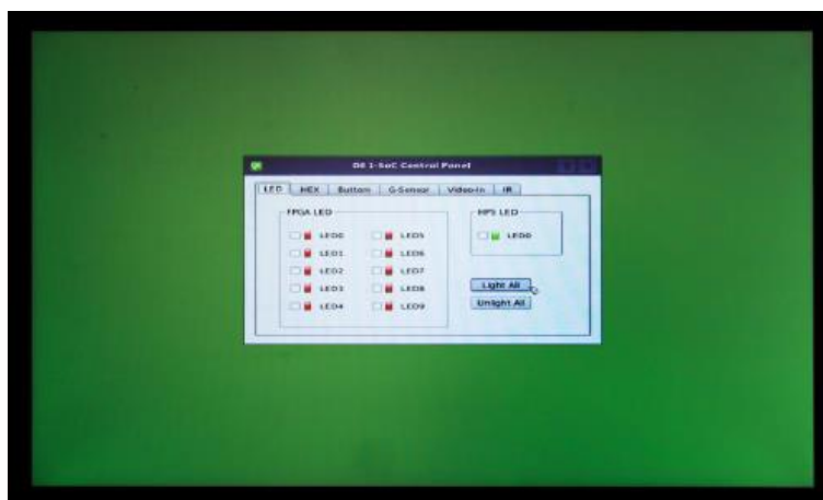
Figure 7-4 Screenshot of DE1-SoC Control Panel
