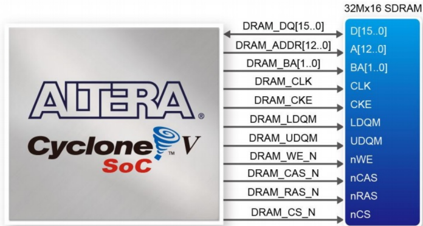
Figure 3: 64MB SDRAM FPGA Interface
