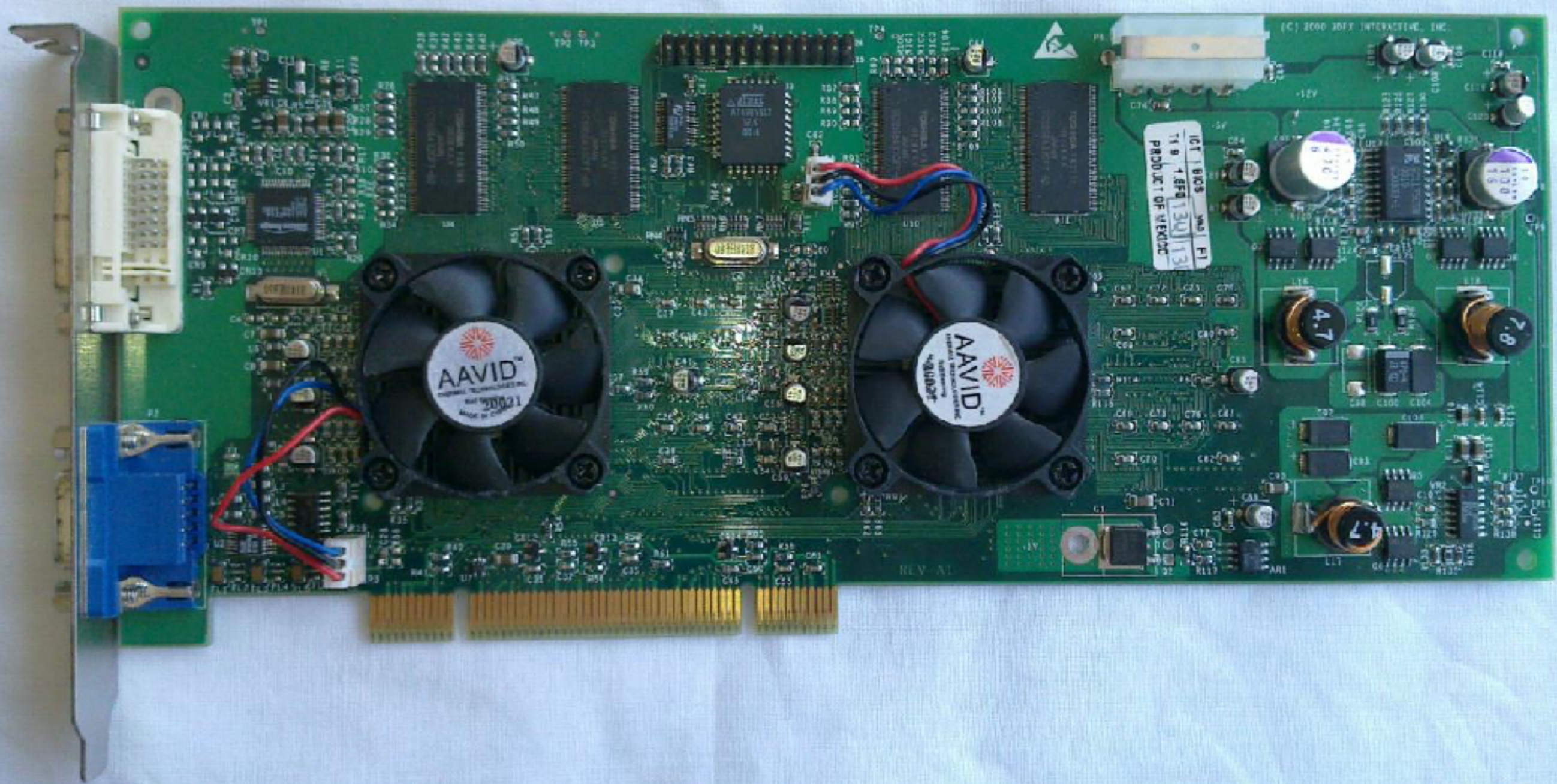
3Dfx Voodoo 5 1999 Note fans & auxiliary power connector
