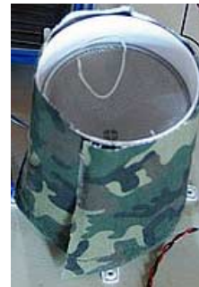
Fig. 6. Camouflaged Rainfall Sensor
