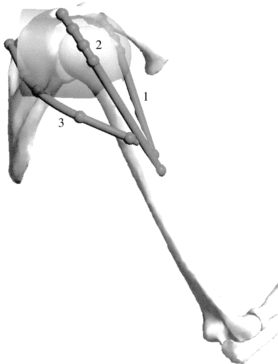
FIGURE 6 Posterolateral view of the obstacle-set model used to represent the paths of the three heads of deltoid. The anterior head (1), middle head (2), and posterior head (3) are each modeled using a sphere-capped cylinder obstacle set. Only the obstacle-set used to model the middle head (2) is shown. The paths of the three heads are modeled using different sizes, positions, and orientations for the obstacles. The locations of the attachment sites of the muscle and the locations and orientations of the obstacles were chosen to reproduce the centroid paths of each head. The geometry of the bones and centroid paths of the muscles were obtained from three-dimensional reconstructions of the anatomical structures.
