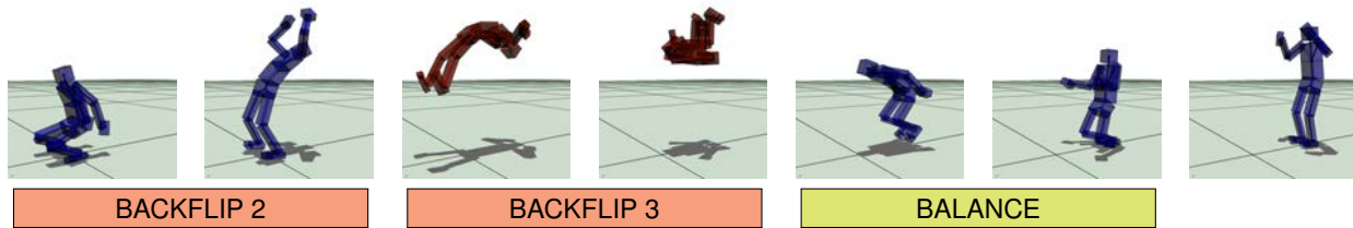
Fig. 8: The backflip is produced by controlling COM height, contacts, and maximizing angular momentum. The first and middle frames of windows 2 to 4 are shown, together with the final frame.
