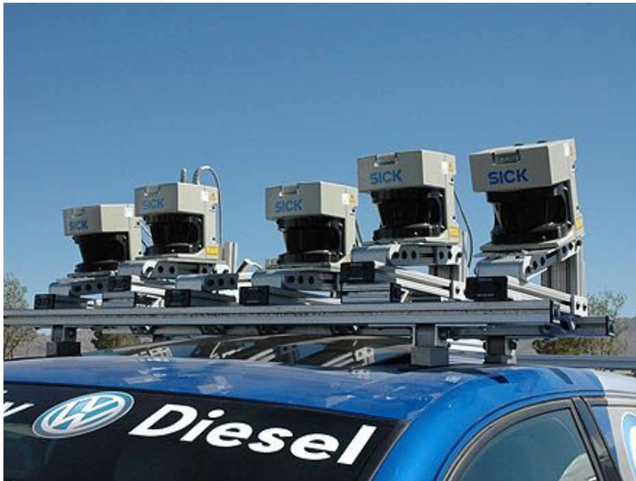
5 SICK lasers for mapping and localization on the 2005 winning VW Touareg "Stanley"
