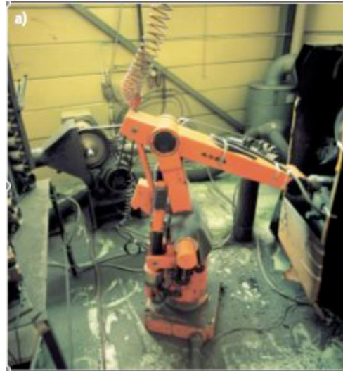
ASEA IRB-6 (1973) first robot all-electric-drives
