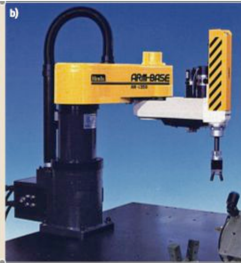
Hirata AR-300 (1978) first SCARA robot
