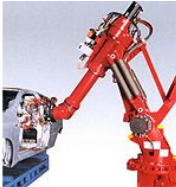
Comau Smart H4 closed kinematic chain
