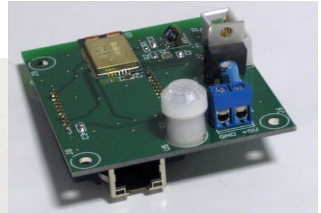
Ceiling PIR 802.15.4 bridge
