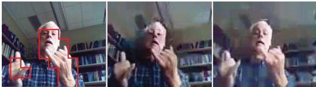
Figure 3.8: A snapshot of ROI-based Encoder (a) original frame with skin blocks (red lines) (b) 0 ROI (c) 12 ROI. The quality in skin blocks is enhanced while the quality in the rest of blocks is degraded.
