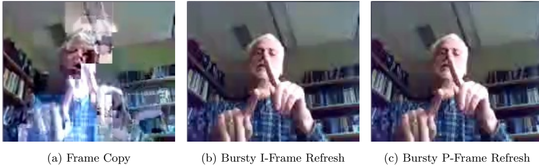
Figure 4.1: Visual comparison of recovery techniques. Figure shows frame number 325 of the test sequence.
