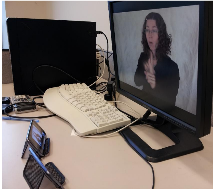
Figure 37: Experimental setup where two Samsung Galaxy S3 phones are facing a computer screen with a video of a woman signing in ASL.
