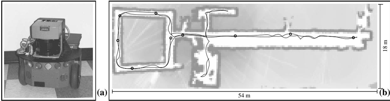
Fig. 2: a) Pioneer II robot used throughout the experiments. b) Map used for localization along with the path followed by the robot during data collection. The small circles mark the different start points for the global localization experiments.
